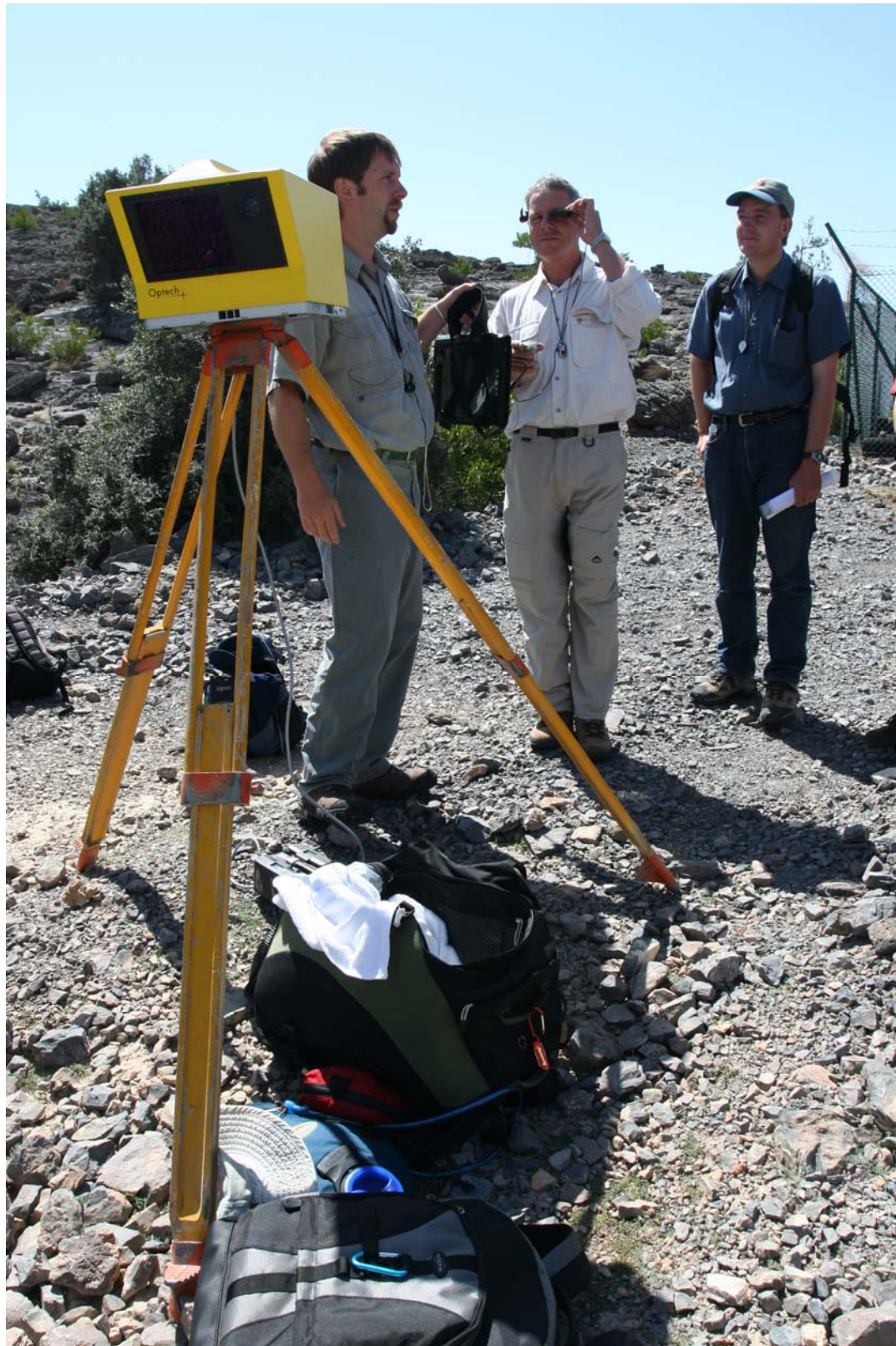
Lidar scanning and head-mounted display allow data processing and interpretation directly in the field.
